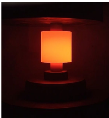
Fig. 12 Image of the graphite press in the vacuum chamber during the Cr powder sintering
