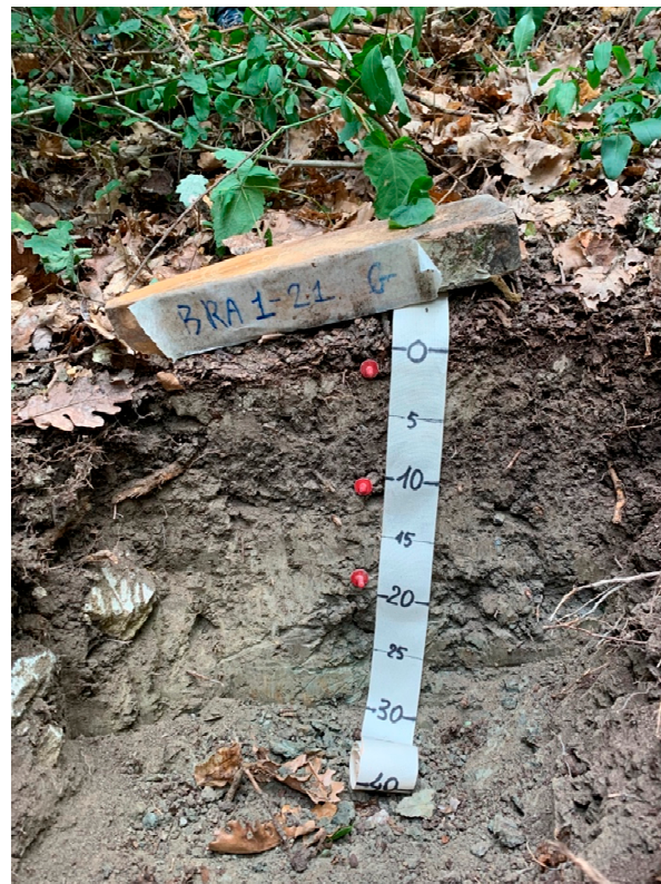
Figure 2. Sampling soil layers (0–15 cm and 15–30 cm) from a minipit dug at one of the farms investigated by the SuoBo project.
