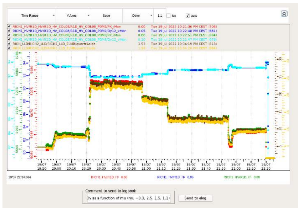
Figure 4.56: Trends of the July \mu scan. The last dynode was not powered yet. The variable more sensitive to the luminosity variation is I_{PK} (PK_imon in the legend). The voltage of the last dynode exhibits a drop of \sim 2 V at the highest luminosity reached in the scan. The voltages and currents are shown for 2 PDMs in the central region of RICH1. Also, the currents from the LLD detector positioned in RICH2 see the light from the pp collisions, as shown in the brown and yellow lines.
