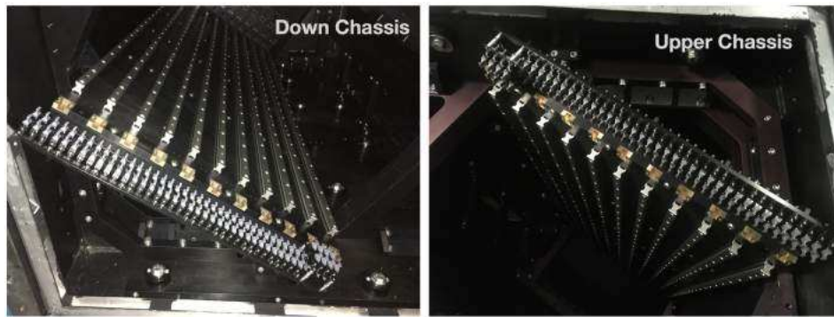
Figure 3.12: Support structure for the RICH1 columns, the MaPMT chassis, showing the rails and alignment structures. The chassis is mounted to the soft-iron magnetic shielding that surrounds the MaPMT region.
