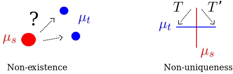
Figure 3.1: (left) Example of a case in which a solution for the Monge problem does not exist. (right) Example of a case in which the solution for the Monge problem is not unique.
