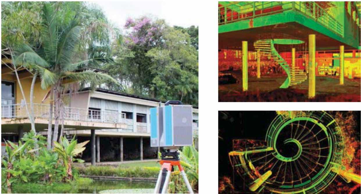
Figure 1.7: Olivo Gomes House by Brazilian architect Rino Levi: 3D survey pilot project and first elaboration of external stairs from point cloud images.
