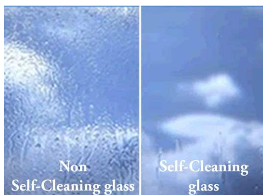
Fig. 16 – Difference between a non-treated glass and a glass with self-cleaning treatment.
