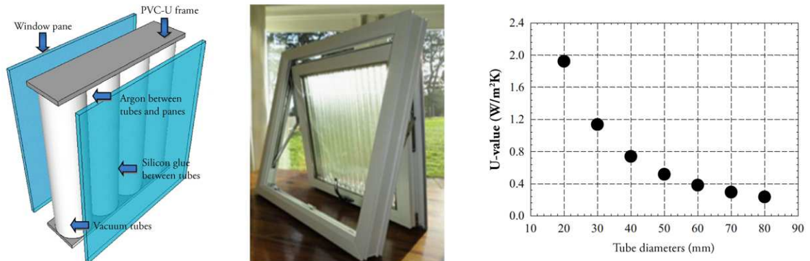
Fig. 46 – From left to right: Scheme of the Vacuum Tube Window glazing; Sample realized at the University of Nottingham; Relationship between tube diameters and system's U-Value.
