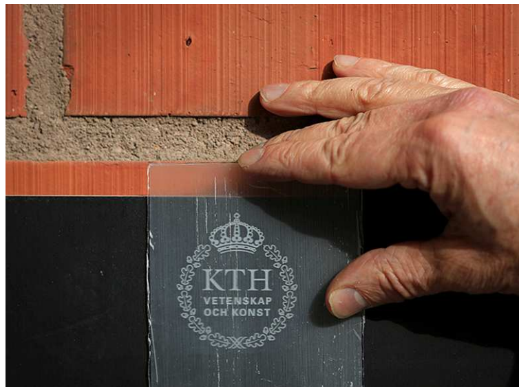
Fig. 04 – Translucent wood developed within the KTH Royal Institute of Technology in Stockholm.
