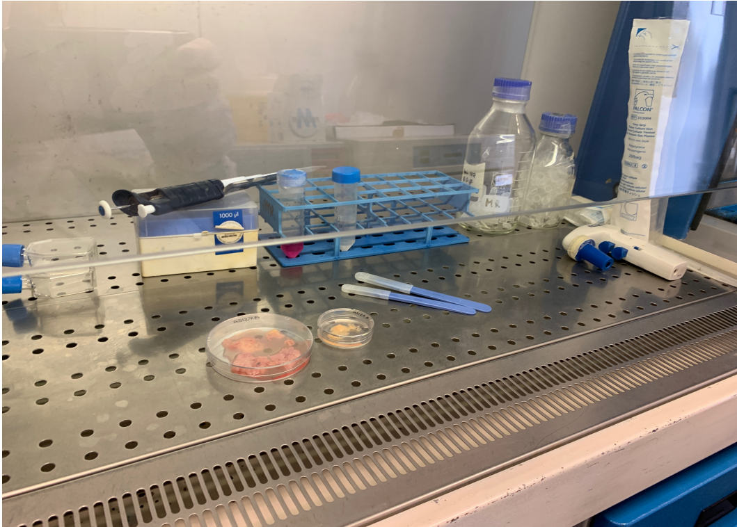
FIGURE 3.1: Laminar flow hood in laboratory of medical genetic, to preserve the sterility of the sample
