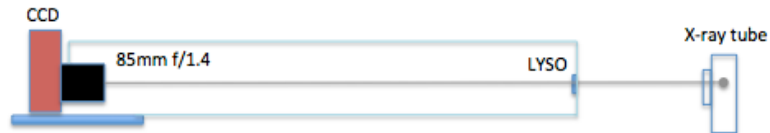
Figure 4.1 - Sketch of the experimental setup used to test the GPI prototype
