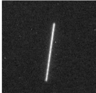
Figure 4.6 - Slit camera image acquired with aperture f/1.4 and exposure time of 2 seconds
