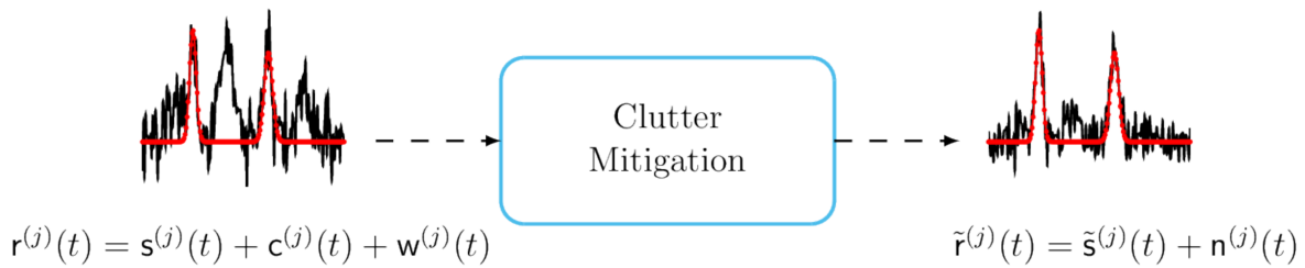
Figure 6.1: Pictorial representation of the clutter mitigation filter. Signals in input are defined in (6.1) and represent the components relative to the target, clutter, and thermal noise, respectively. Signals in output are defined in (6.9) and represent the component relative to the filtered target component and clutter-plus-noise, respectively.
