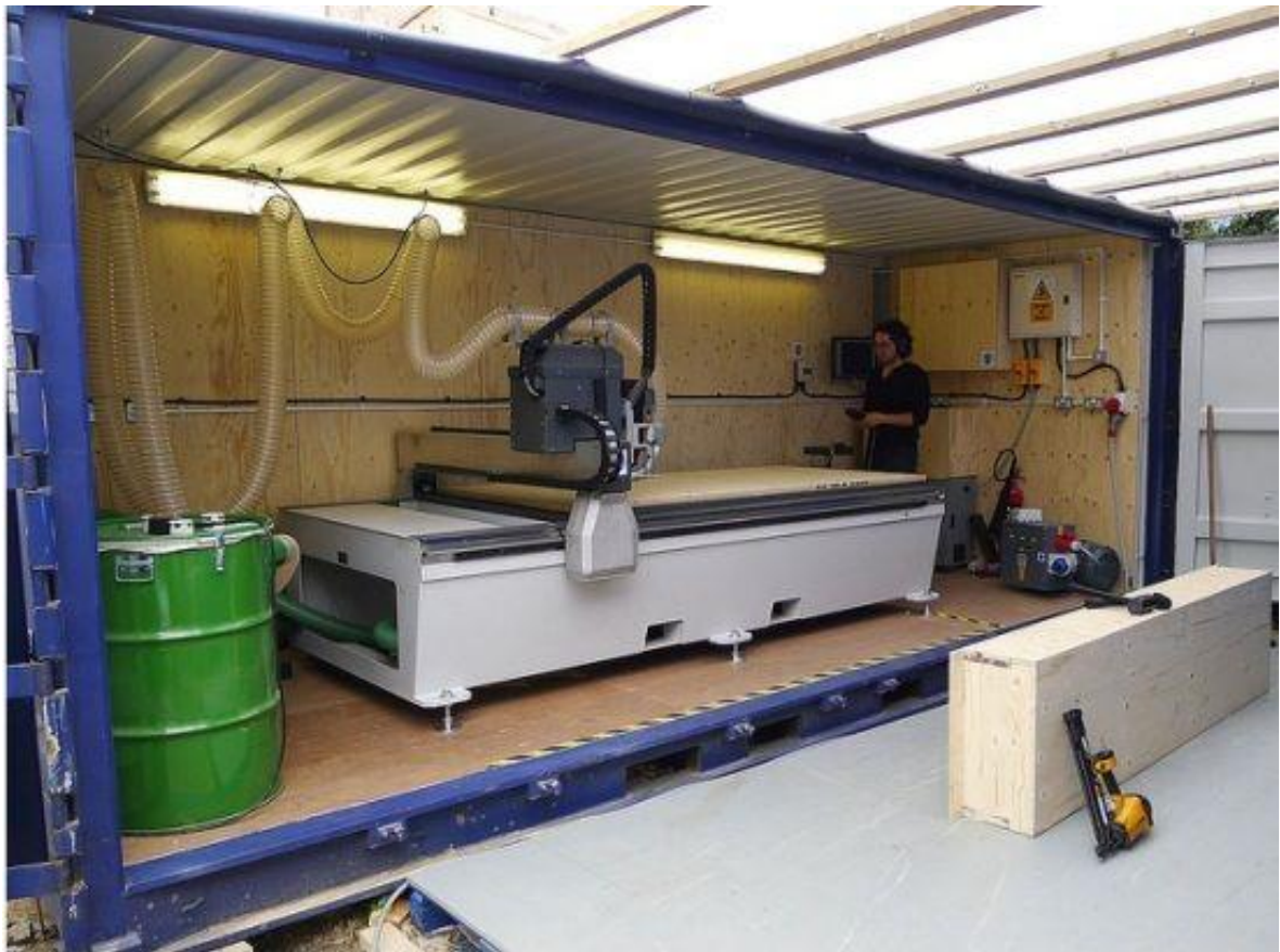
Figure 41 On-site fabrication CNC router created by FACIT homes. Credits: FACIT Homes
