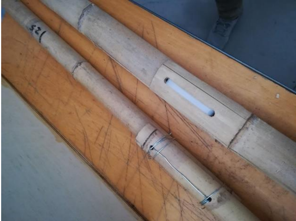
Figure 86 Overlapping bamboo connections for Vertical elements tried with zip ties and metallic wire, photo: author (2018)
