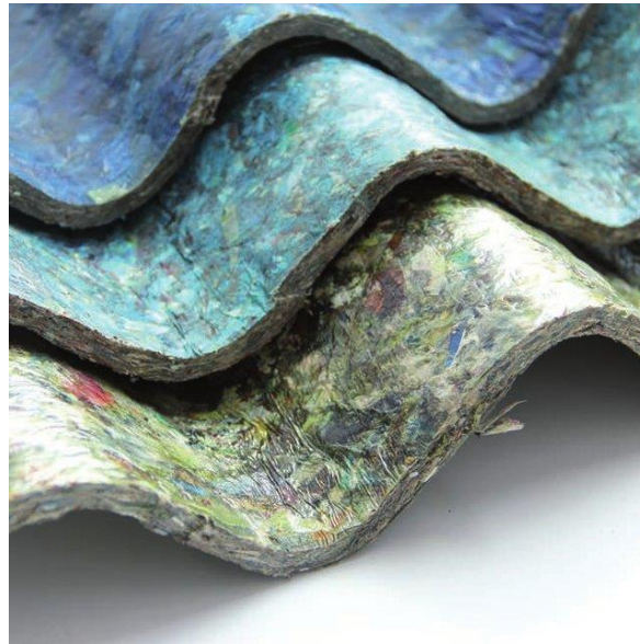
Figure 25 Tuff Roof - a corrugated roofing material made out of reclaimed Tetra Pak packaging. Source: Building from Waste (2015)
