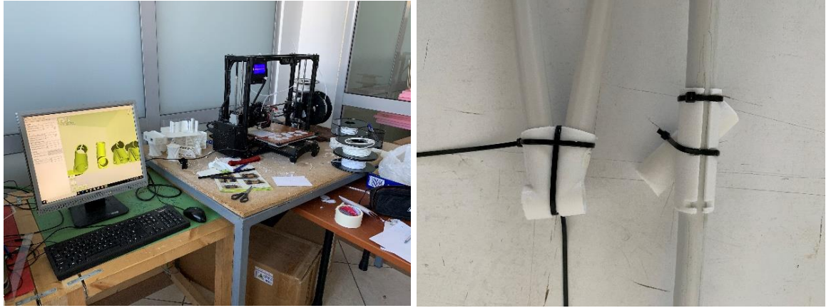
Figure 103 Joints being prepared for 3-D printing in the Polis Lab (a), Testing the joints ease of assembly through friction (b) Photo: Sara Codarin
