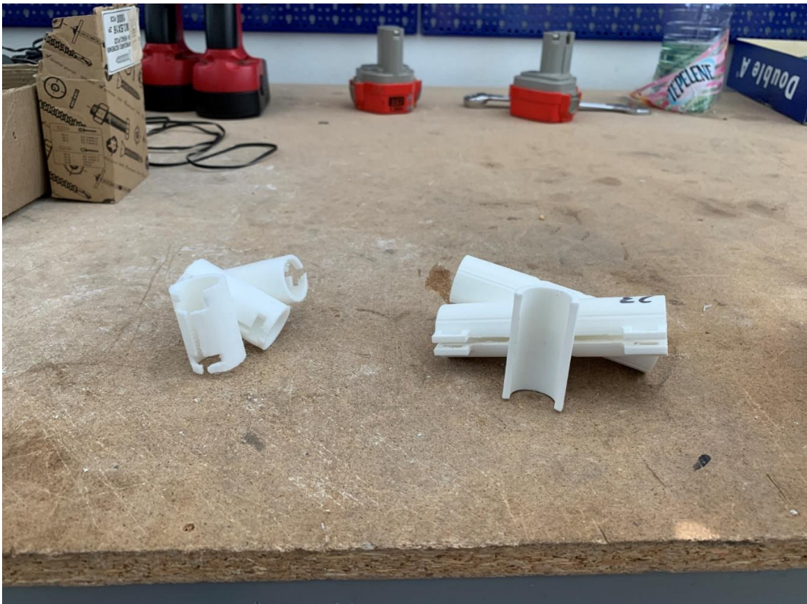
Figure 104 Joint difference from last to first printed joints. Thickness and length of joints were reduced. Photo: author
