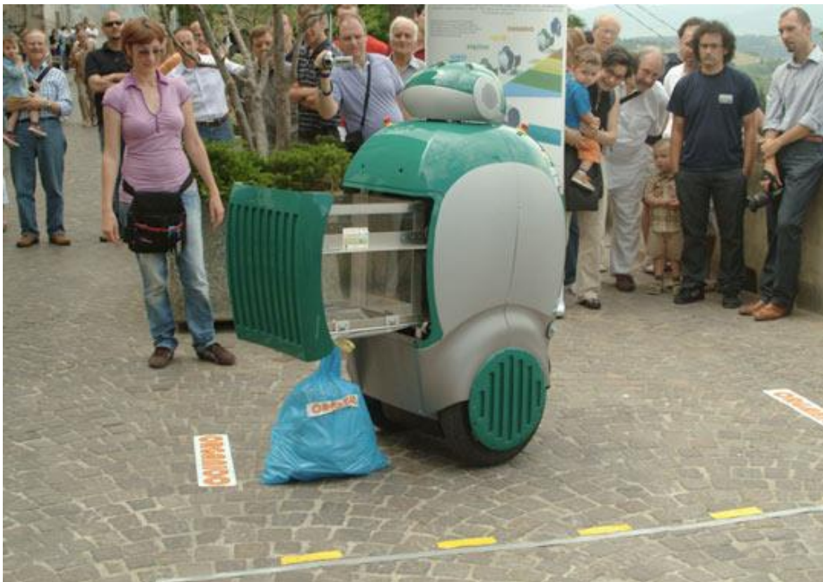
Figure 53 The DustCart Robot, an autonomous service robot designed to collect waste door-to-door. Photo: inhabitat.com
