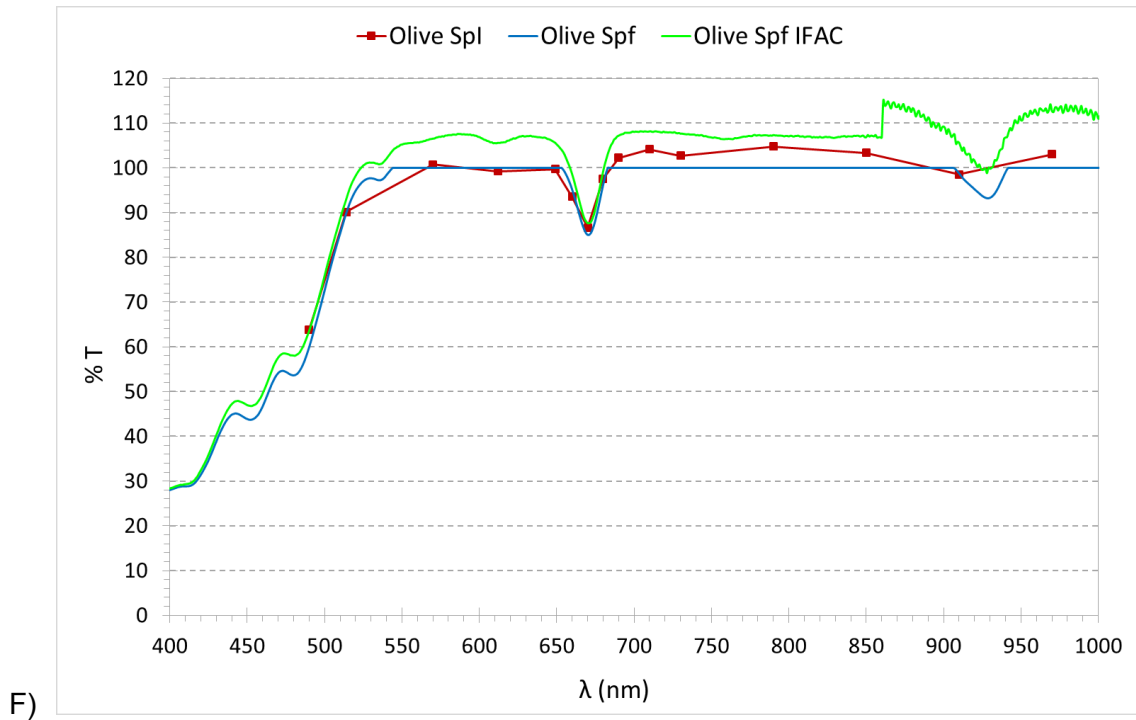
F) FIGURE 78 – COMPARISON OF TRANSMITTANCE SPECTRA OBTAINED WITH IMAGE SPECTROSCOPY (SPI), SPECTROPHOTOMETERS LAMBDA 25 (SPF) AND LAMBDA 19 (SPF IFAC) FOR THE SAMPLES A) LECCINO, B) CORATINA, C) FS17, D) LAMPANTE, E) REFINED OIL, F) OLIVE OIL
