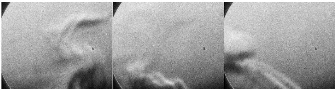
FIGURE 54 – DISPLAY OF THE HEAT “PLUME” FROM THE TIP OF A WELDER. EACH PLUME IS DOUBLE BECAUSE OF ITS REFLECTION ON THE MIRROR
