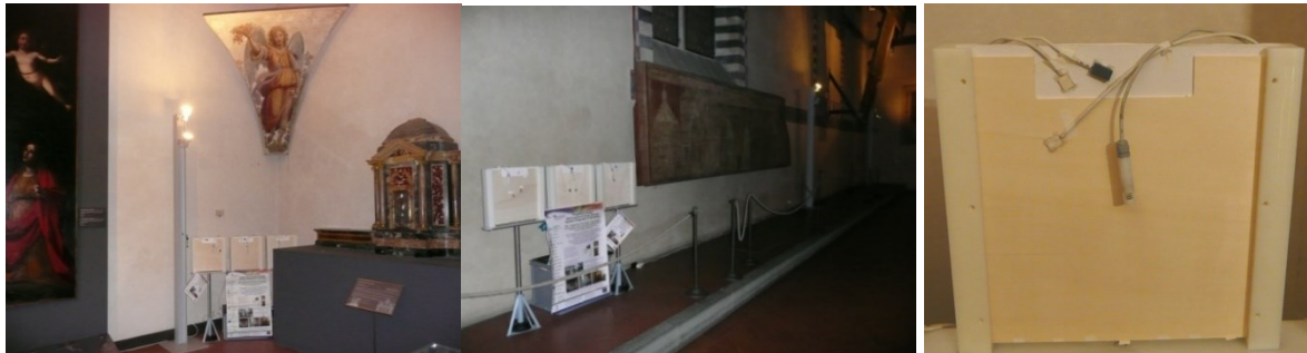
FIGURE 9 - PCMs TESTING IN ROOM I AND VI OF THE SANTA CROCE MUSEUM AND MICROCLIMATIC SENSORS INSTALLED ON EACH PANEL
