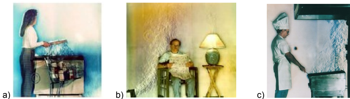
FIGURE 39 - FULL-SCALE SCHLIEREN PHOTOGRAPH TRIALS. A) A SHOPPER REMOVING A FROZEN PIZZA FROM A CHEST-TYPE GROCERY STORE FREEZER; B) A DOMESTIC ROOM WITH PERSON, LAMP AND ELECTRIC SPACE HEATER; C) A COMMERCIAL KITCHEN GRIDDLE AND EXHAUST HOOD IN USE WITH COOKING FUMES (SETTLES G.S., 1997)
