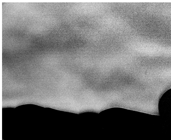
FIGURE 57 – IMAGE OF THE HEAT TURBULENCE FROM THE HAND, ELABORATED BY SUBTRACTING THE BACKGROUND (“WHITE FIELD”, FIGURE 56-B) TO REMOVE THE SPOTS AND ADJUSTING BRIGHTNESS/CONTRAST TO EMPHASIZE THE STRIKES
