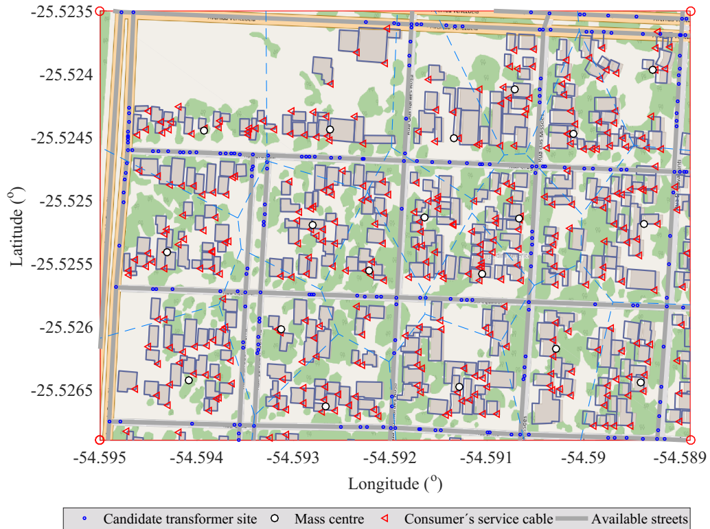
Figure 3.2: Studied scenario showing the transformer candidate location, in every corner in the map.
