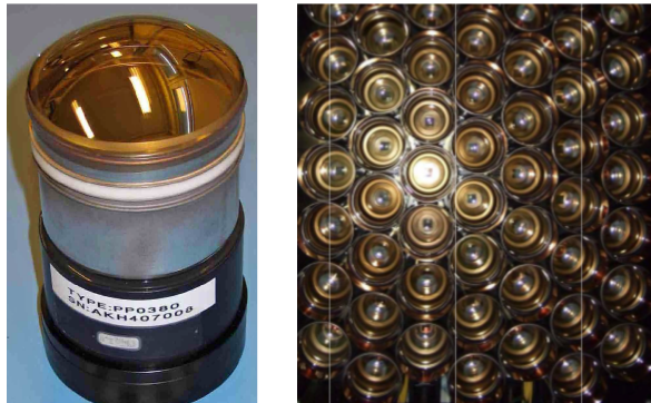
Figure 3.4: Image of a single HPD (left) and the RICH1 HPD plane (right) [62][96].
