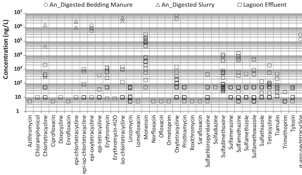
Fig. 13. Occurrence of antibiotics in different types of treated liquid/semiliquid cattle manure. Data from: Arikan (2008), Arikan et al. (2006), Hafner et al. (2017), Watanabe et al. (2010), Zhang et al. (2013).
