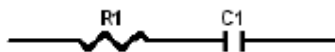
Fig.8.4 Simple electrical circuit composed by a resistor (R) in series with a capacitor (C).
