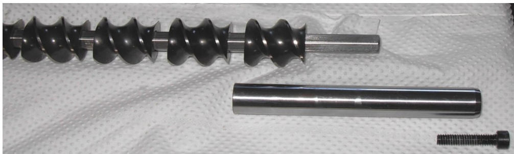
Figure 2 43 Estrusore bivate Twin-Screw Extruder type LTE-26-40: vite modulare
