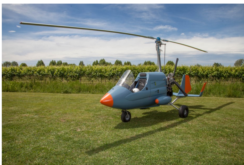
Figure 1.1. Picture of the Radgyro, the autogyro dedicated to multispectral airborne acquisitions, used for the AGRS surveys over the sea
