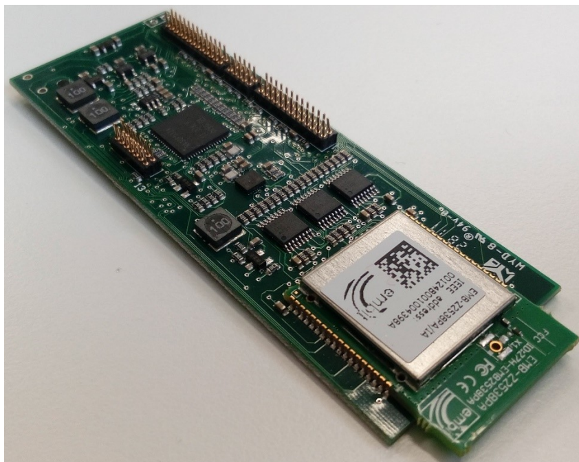
Figure 22. Prototype of wireless sensor network node suitable for safety related applications
