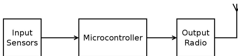
Figure 18. WSN node typical architecture.
