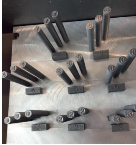
Figure 2.2. Building platform with the L-PBF produced cuboid and tensile specimens.
