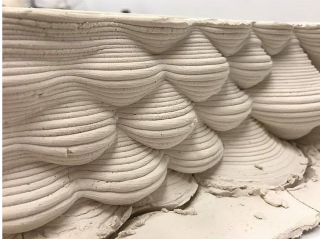
Figure 29 - Early attempts at hand control of clay flow rate
