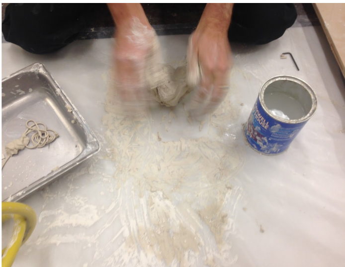
Figure 28 - Mixing clay Prior to printing
