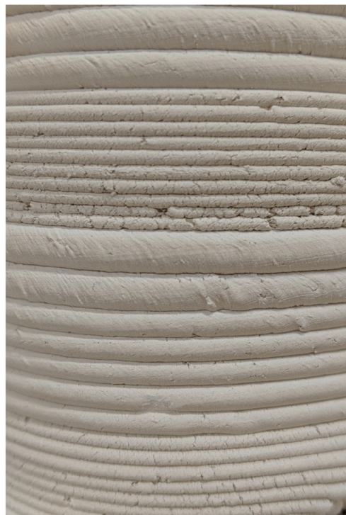
Figure 44 - Varying Layer Height
