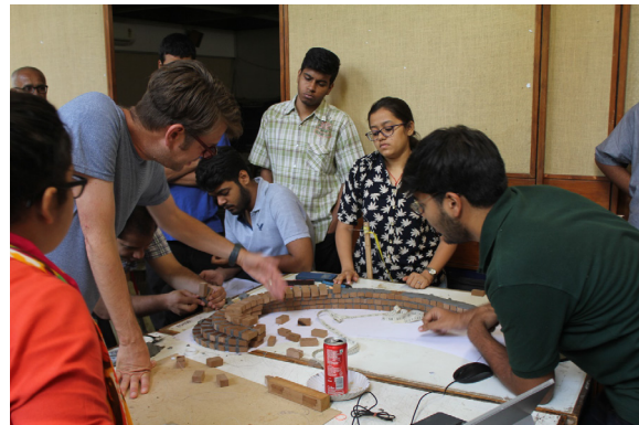
Figure 10 - Students testing scaled models using wood blocks and clay to represent the bricks and mortar
