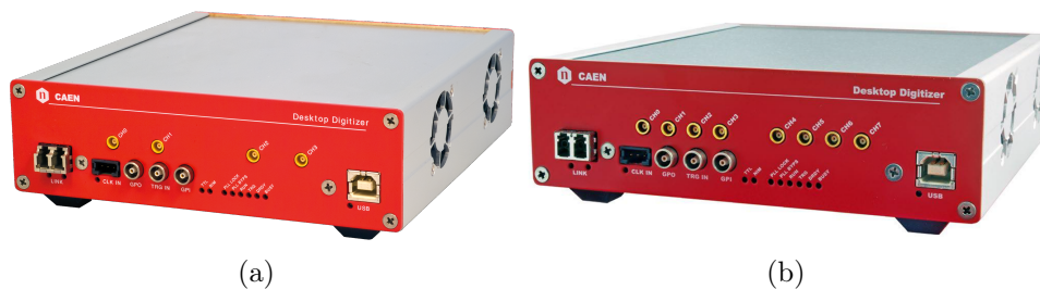
Figure 4.12: Front view of the CAEN desktop digitizers employed in the experiment: a) DT5751; b) DT5730SB [69].
