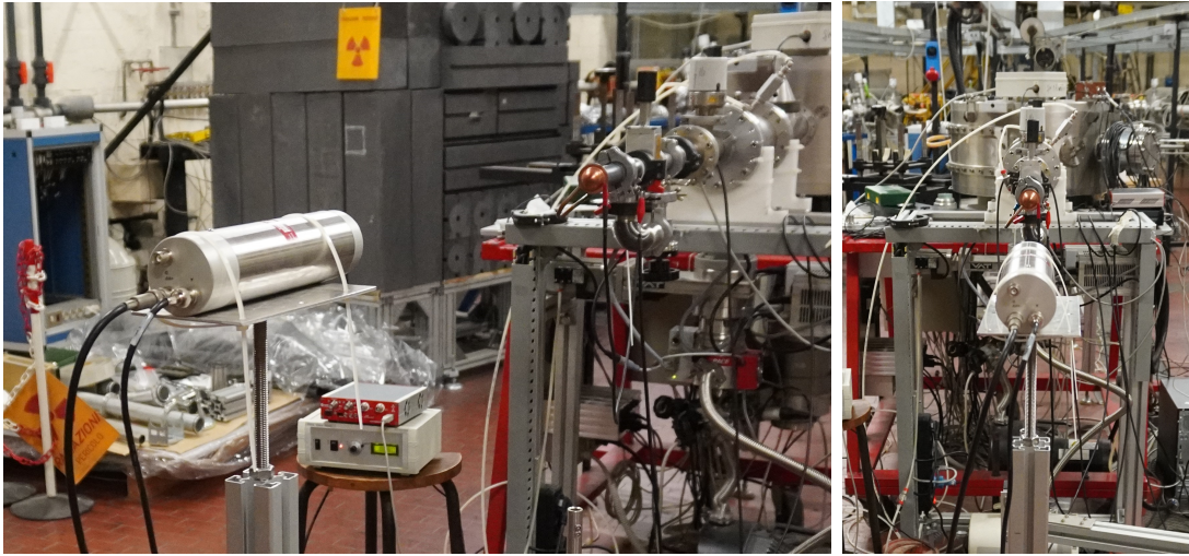
Figure 5.1: Experimental setup for neutron time-of-flight measurement with a proton energy of 1912 keV from two different points of view. Detector located at 71.99 \pm 0.01 cm from the target at zero degrees relative to the beam direction.
