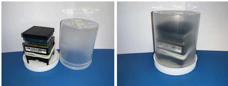
Figure 8.38: The H-type EC screwed to the plastic jar cap ready to be sent to CERN. The barcode is visible on its side and a label with the EC load number and the station used to test it is placed on the jar bottom, which is facing upwards.
