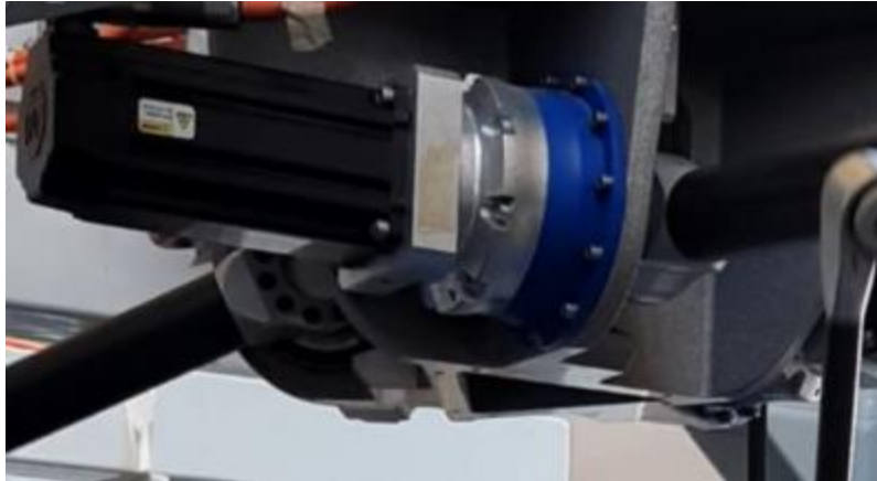
Figure 6.2 - Kinetix VP Motor used in CT Flex robot.
