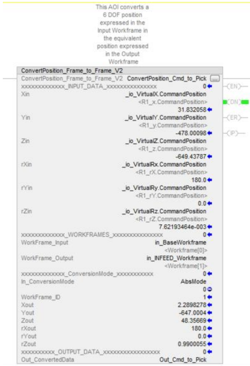
Figure 7.9 - Converting a given position from one frame to another in Logix Designer.
