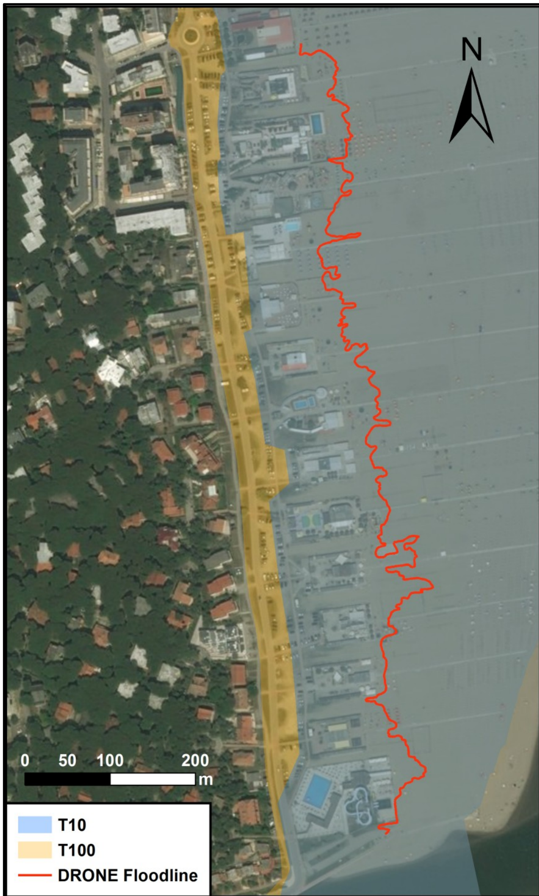
Figure 2.9 Comparisons between the observed "DRONE Floodline" and the flood scenarios (T10 and T100) computed by Perini et al. (2016).
