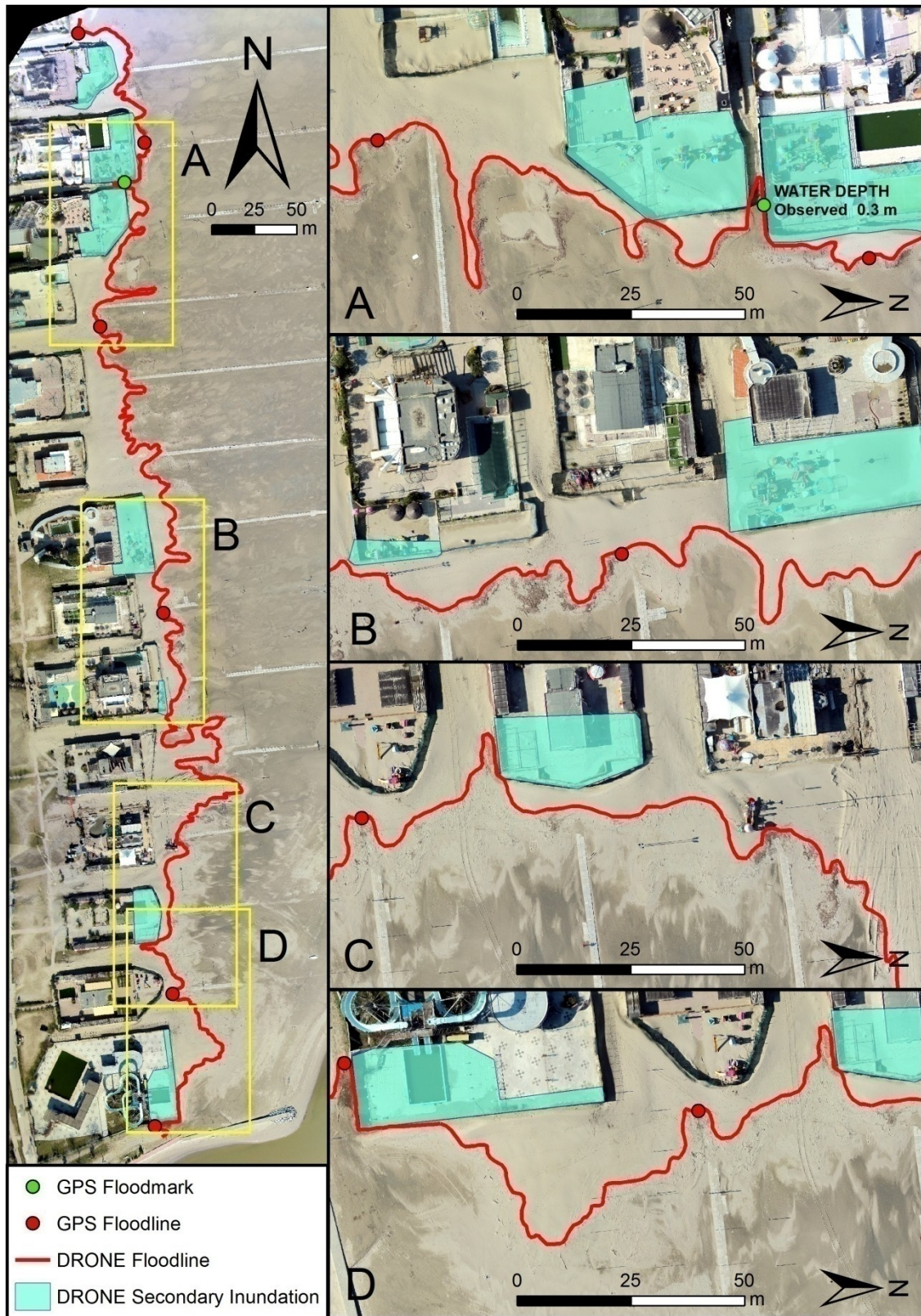
Figure 2.7 Observed “GPS Floodline” and “GPS Floodmark” (green and red circles), drone (red solid line and light-blue polygons) flood extension comparisons: the box on the left shows an overview of the target area while on the right (A, B, C and D) some spot-focuses are given.
