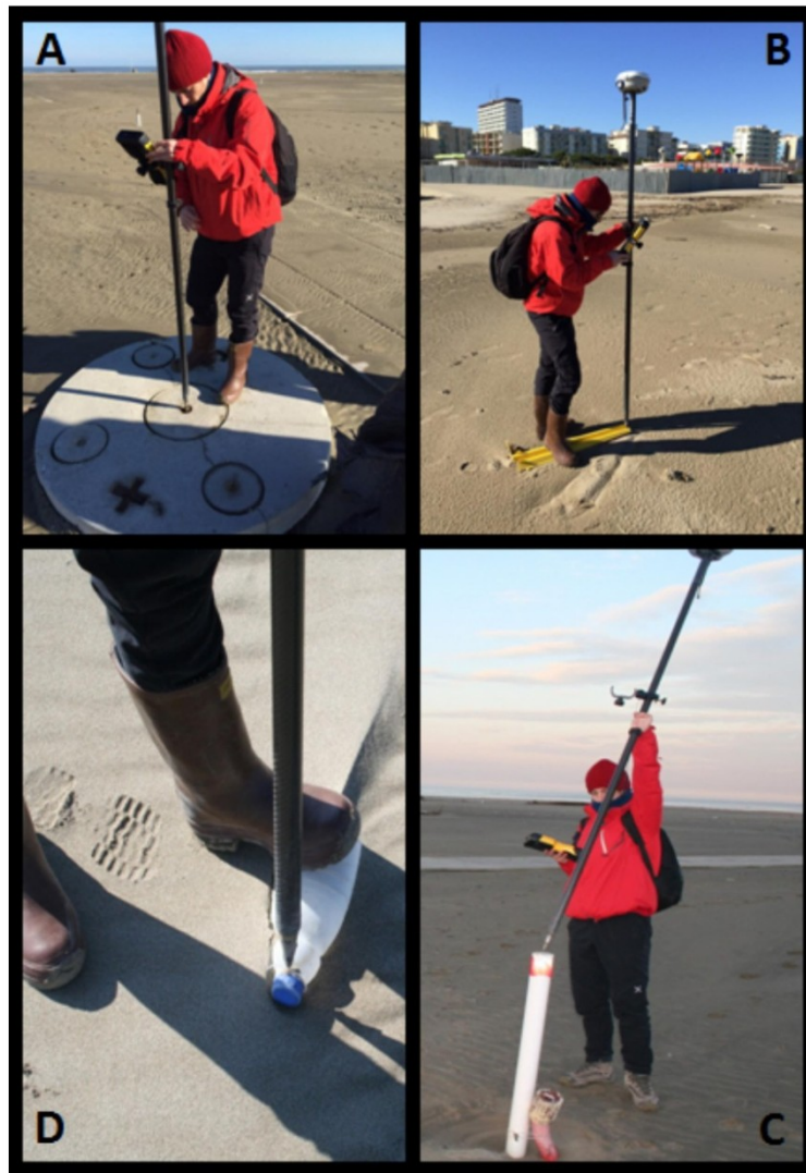
Figure 2.10 Photos A and B at the top demonstrate practical GCPs based on unique shapes, colours, and ability to see from a high altitude. Photos C and D, on the bottom, demonstrate error-inducing GCPs due to their height off the ground and indistinguishable shape, size, and colour in aerial images.
