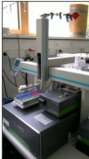
Fig.19 Instrument Picarro L2140, used in TU Darmstadt, automatic sampling device.
