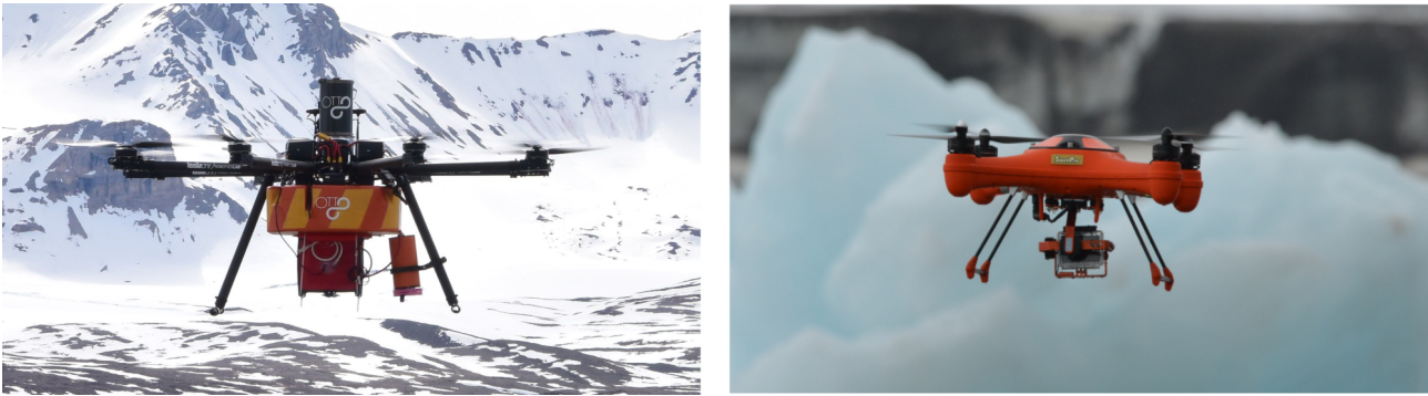
Figure 3.7. On the left there is OTTO UAV with the AirQino (red box) and the Thermal Camera (orange box) mounted on-board. On the right the Splash UAV is shown.
