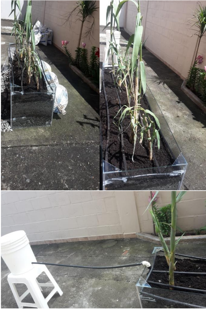
Figure 18 Pilot VSSF CW
