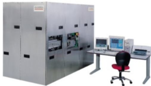
Figure A.3: SIMS Cameca SC Ultra/Wf, present at Bruno Kessler Foundation laboratories.
