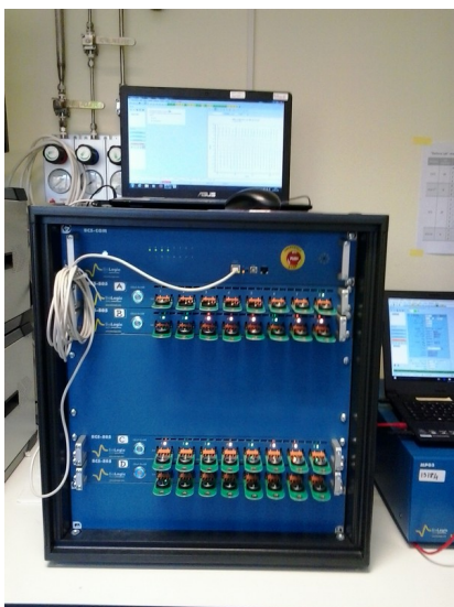
Figure 3.3: BioLogic BCS-805 used to test coin-cells.
