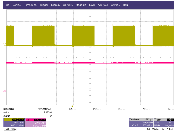
Figure 4-12: Class-E converter with backward communication channel used to regulate the output voltage. Yellow: main clock signal V_g showing on-off converter modulation; Red: regulated output voltage V_{out}
