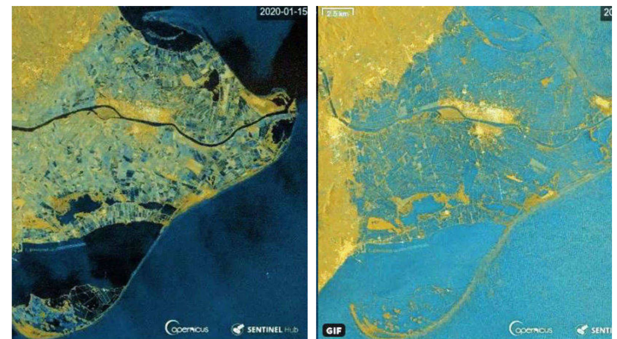
Fig. 9. Flood in Deltebre (Spain), 2019. Marine ingresson reached 3km inland, covering by flood the areas with critical topography. This events caused several damaged and some victims. source: ESA and Copernicus
