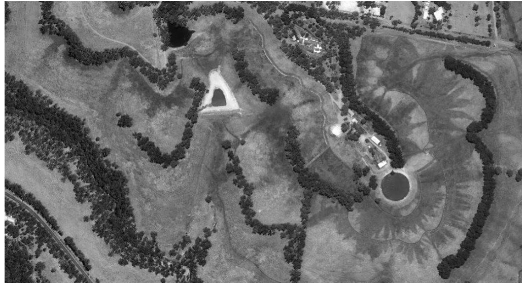
Fig. 118. Nevallan (Australia). Nevallan in summer, you can see the wetter areas well thanks to the “keyline”. If you look closely you will notice that the wettest point is not necessarily the valley. source: www.permacultu-raincorso.it Keyline design is a landscaping technique of maximizing the beneficial use of the water resources of a tract of land. The “keyline” denominates a specific topographic feature related to the natural flow of water on the tract. Keyline design is a system of principles and techniques of developing rural and urban landscapes to optimize use of their water resources.
