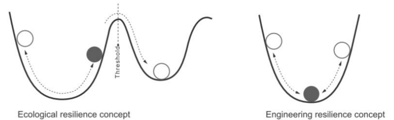
Fig. 50. Difference between engineering and ecological resilience. The cup represents the region in the state space or “basin of attraction”, in which the system tends to remain, and includes all possible values of system variables of interest. The ball represents the state of the system at any given time. source: “A Theory on Urban Resilience to Floods—A Basis for Alternative Planning Practices”, Kuei-Hsien Liao, 2012
