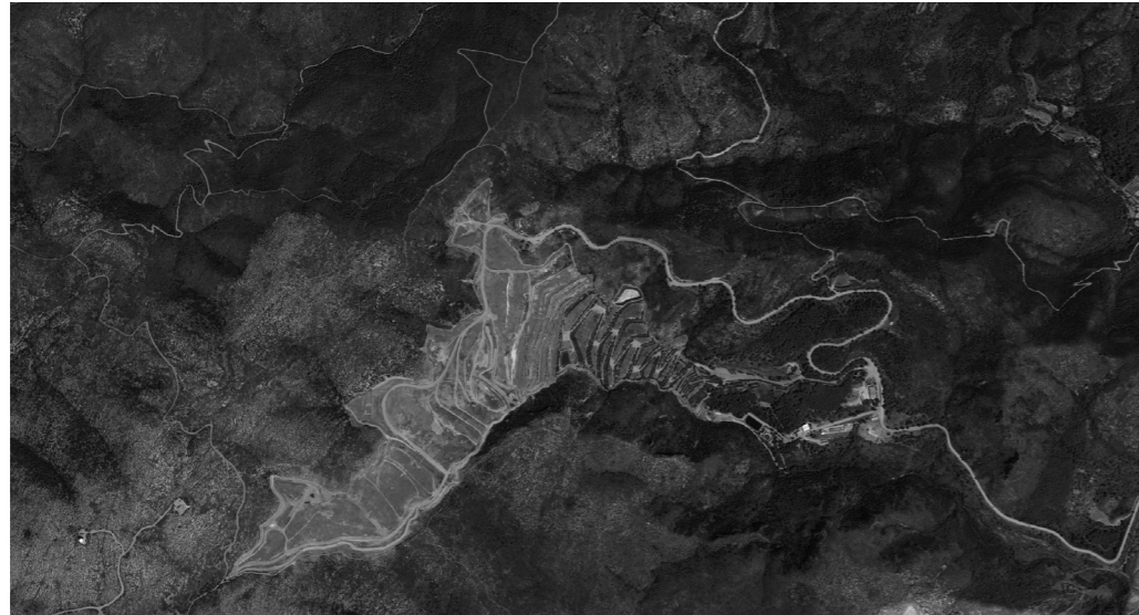
Fig. 109. Vall d'en Joan landfill restoration, Garraff, (Spain) The restoration project defines a pattern of topographic configuration with terraces, side slopes, drainage system, pathways and plantation by phases. source: Google maps
