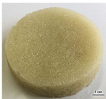
Figure 1. Visual appearance of the wool fibril sponge (wet state). (Courtesy of Dr. Alessia Patrucco)
