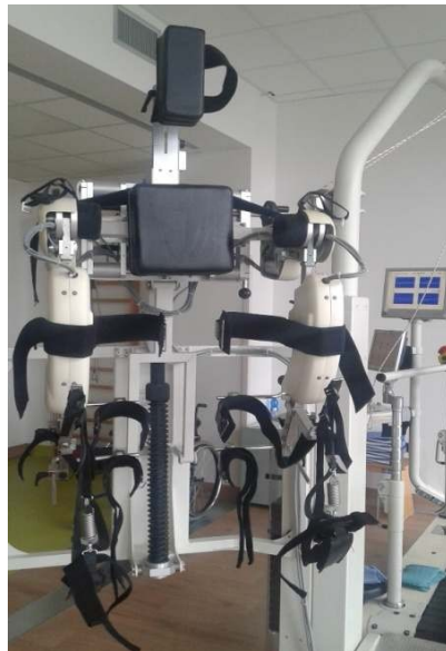
Figure 8. Structure of LOKOMAT (Hocoma Switzerland)
