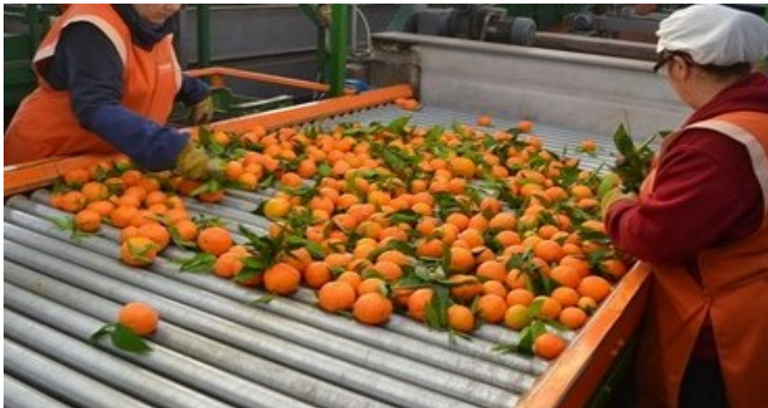
Figure 5a: First inspection on a trash eliminator (originally in colour) (Courtesy: Fresh Plaza)
