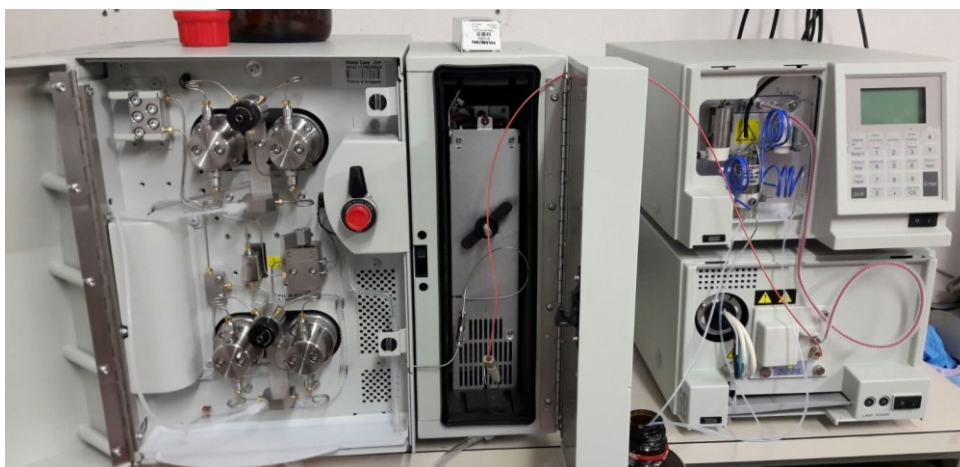
Figure 34: HPLC system (Left: Binary pump and column oven; Right: Detectors) (originally in colour)
