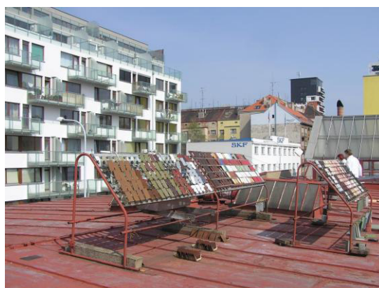
Figure 1.5 Field exposure test of samples within the ICP Materials – Prauge, 2009 ( http://www.corr-institute.se/ ).
