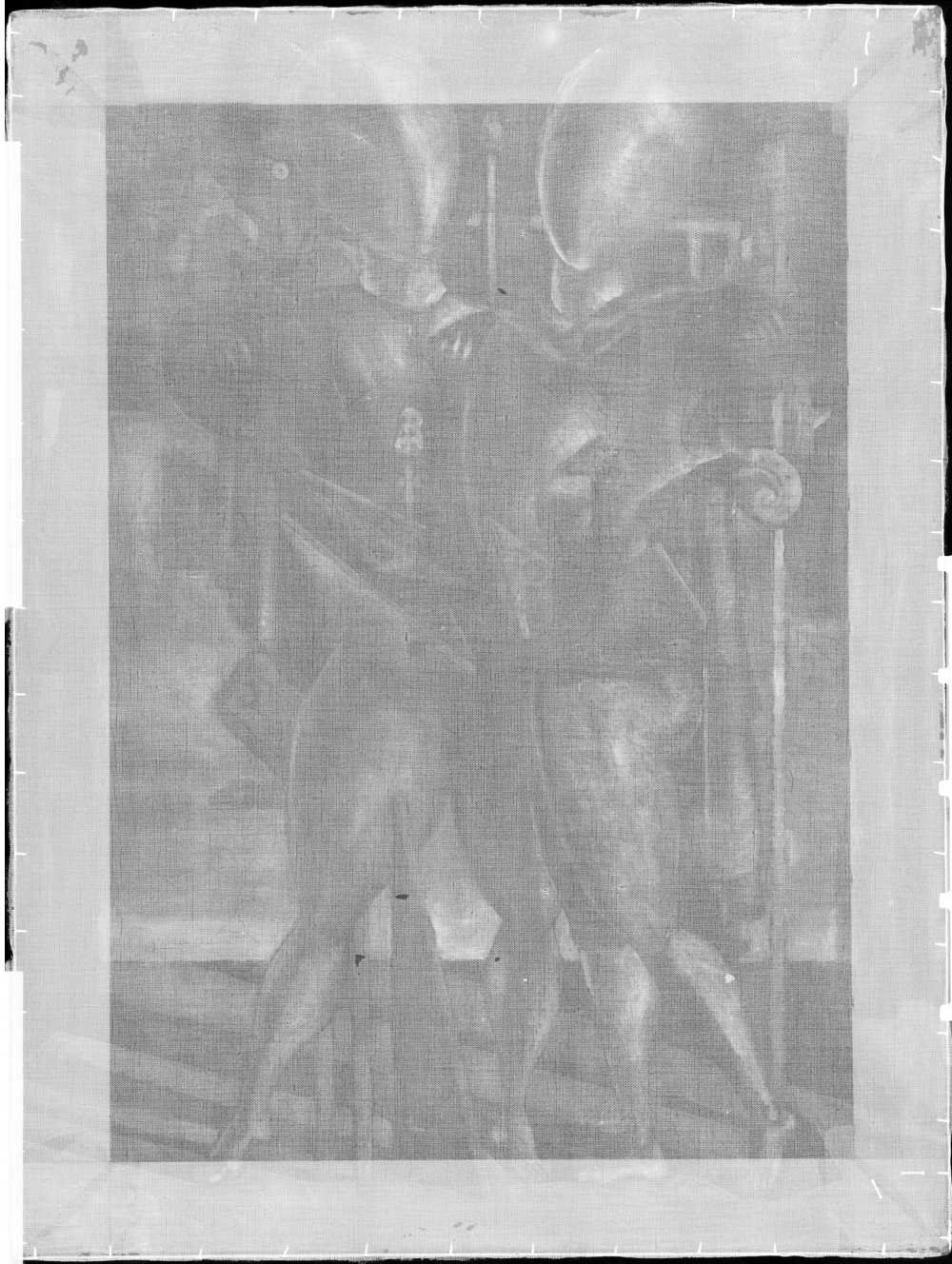
Figure A.17: Radiography of Hector and Andromache composed by 80 images. The W X-ray tube has been set at 20 kV, 19 mA, 0.5 mm of Al filter, 1.5 s time of acquisition.
