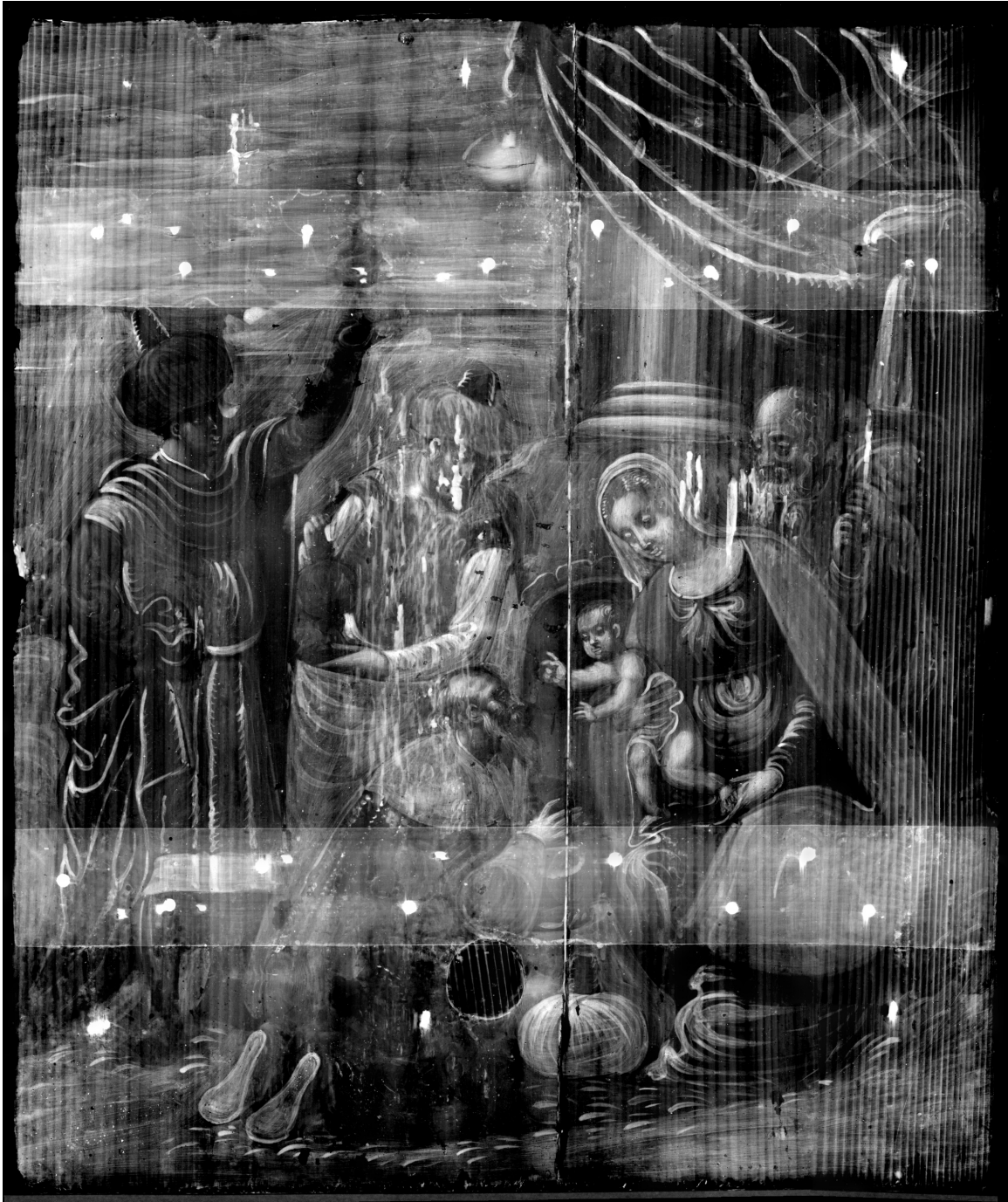
Figure A.7: Radiography of the Adoration composed by images. The Mo X-ray tube has been set at 25 kV, 19 mA, 0.2 mm Al filter, 1.5 s time of acquisition.
