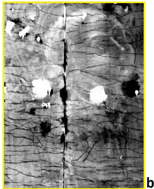
Figure A.2: a) RX of the Virgin and the Child, composed by 58 images, acquired with the Mo X-ray source at 29 kV, 19 mA, 0.18 mm Al filter and 2 s time of acquisition. b) Radiographic detail of the Child's face.
