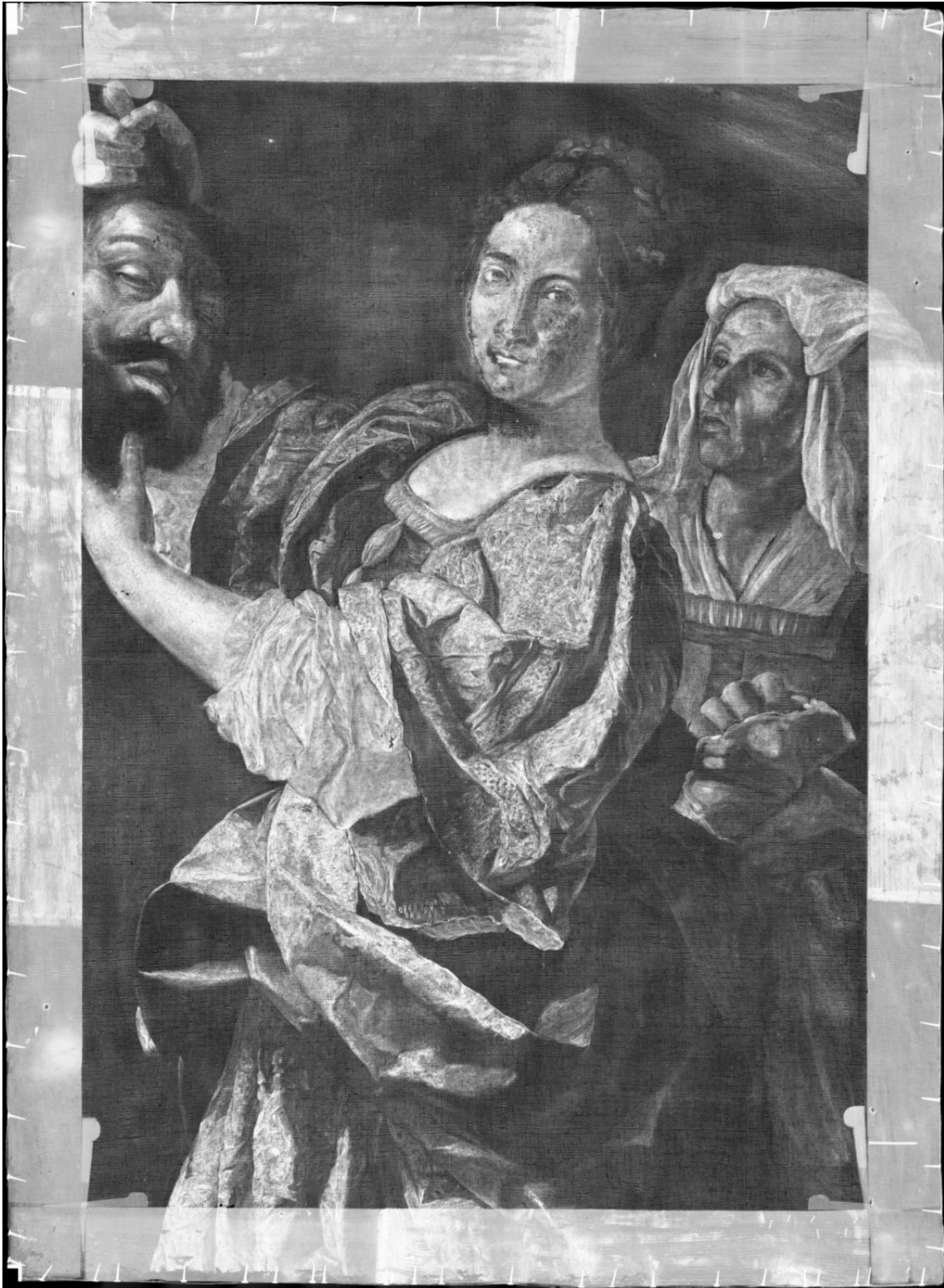
Figure A.9: RX of Judith with the head of Holofernes composed by 266 images. The Mo X-ray tube has been set at 24 kV and 19 mA. The acquisitions lasted 1s.
