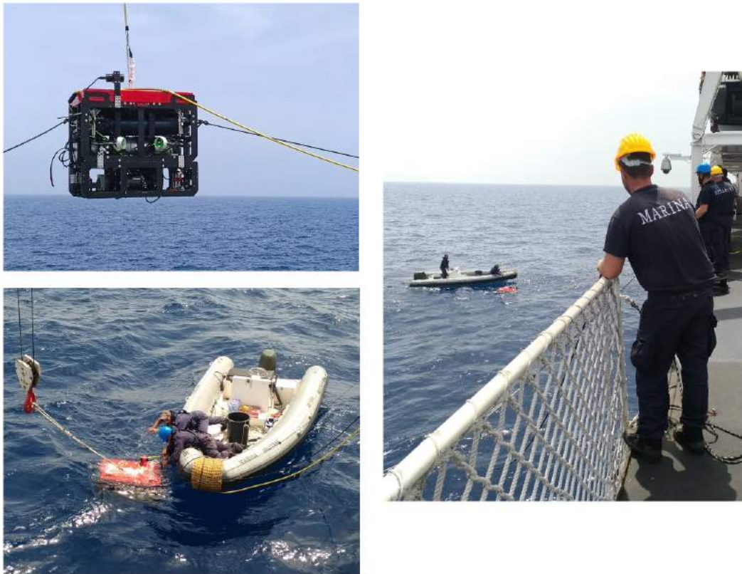
Figure 6.6 – Pictures of e-URoPe during the launching phase from the ITS Magnaghi and of the support operations performed with the rubber dinghy.
