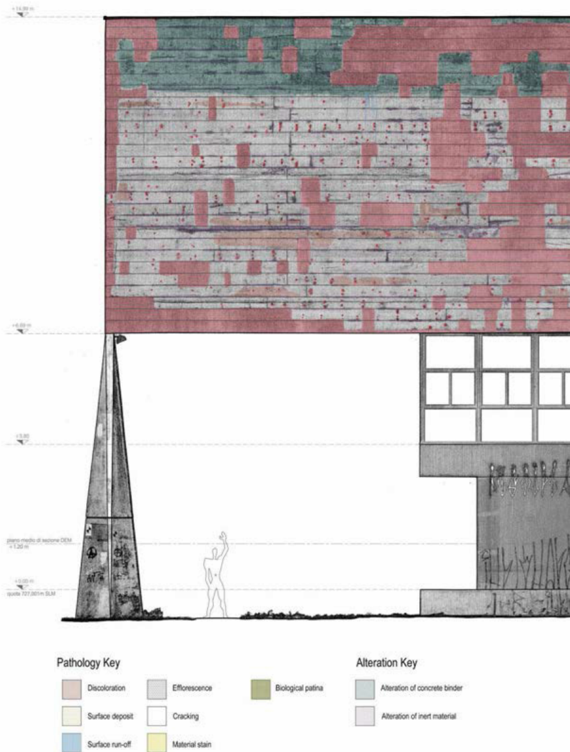
Figure 8.17: FAU USP building, surface analyses identifying main pathologies and materials alteration.
