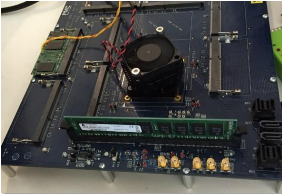
Figure 8.2. SSD controller evaluation board used for interoperability tests. Eight standard SO-DIMM sockets can accommodate NAND flash memory cards, while one standard DDR UDIMM socket can host either DRAMs or MRAM memories.
