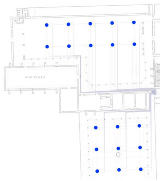
Fig. 8. Arrangement of the BHEs for the case study of “Opera Santa Croce”
