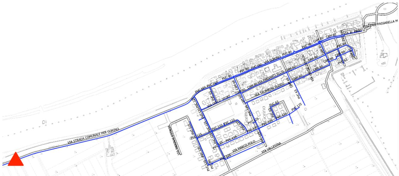
*Figure 1. Layout of the WDN of Gorino Ferrarese (FE). The red triangle indicates the point where the DMA's inlet discharge and pressure are monitored*
