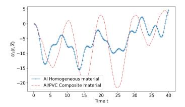
**Figure 9.** Evolution in time of  $U_3(\overline{X}, t)$  at a given point  $\overline{X} = (6.5, 3.5, 0.)$  for a homogeneous Al-plate and an Al/PVC composite plate.
