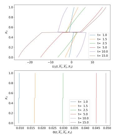
**Figure 6.** Displacement  $U_3$  and temperature  $\Theta$  along the  $X_3$ -axis, on a fiber  $(\overline{X}_1 = 6, \overline{X}_2 = 6, X_3)$ , for given times .
