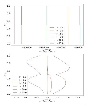
**Figure 8.** Stresses  $\Sigma_{33}$  and  $\Sigma_{13}$  along the  $X_3$ -axis, on a fiber  $(\overline{X}_1=6,\overline{X}_2=6,X_3)$ , for given times.
