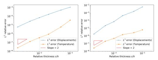
**Figure 4.** Convergence diagrams with respect to  $\varepsilon/h$  for: t = 1 s (**left**); and t = 10 s (**right**).
