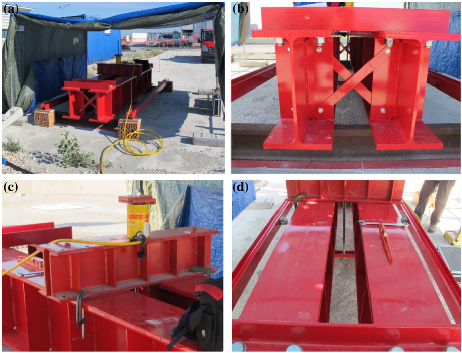
Fig. 10 Test rig for tests on single anchors: a global view; detail views showing b one end section of the reaction frame; c the actuator placed at midspan on the transverse load-transfer beam; d the threaded rod emerging from concrete
