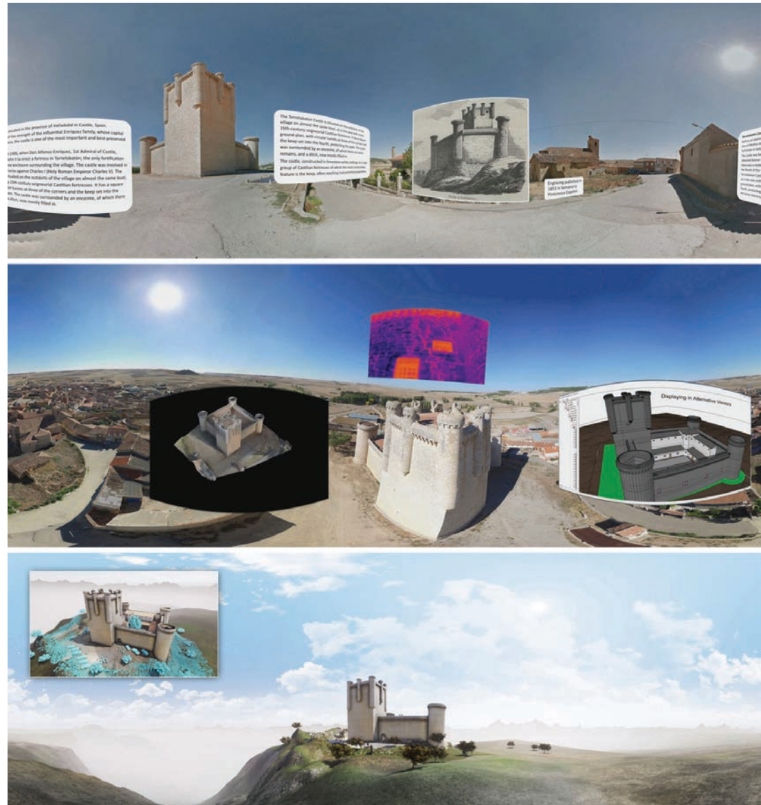
Fig. 9 - The 3D model of the Castle of Torrelabato in Valladolid, Spain, was used to be linked to diagnostic tools, for documentation purposes and for creating an immersive environment, bridging the gap between XR environments for technicians and tourists.
