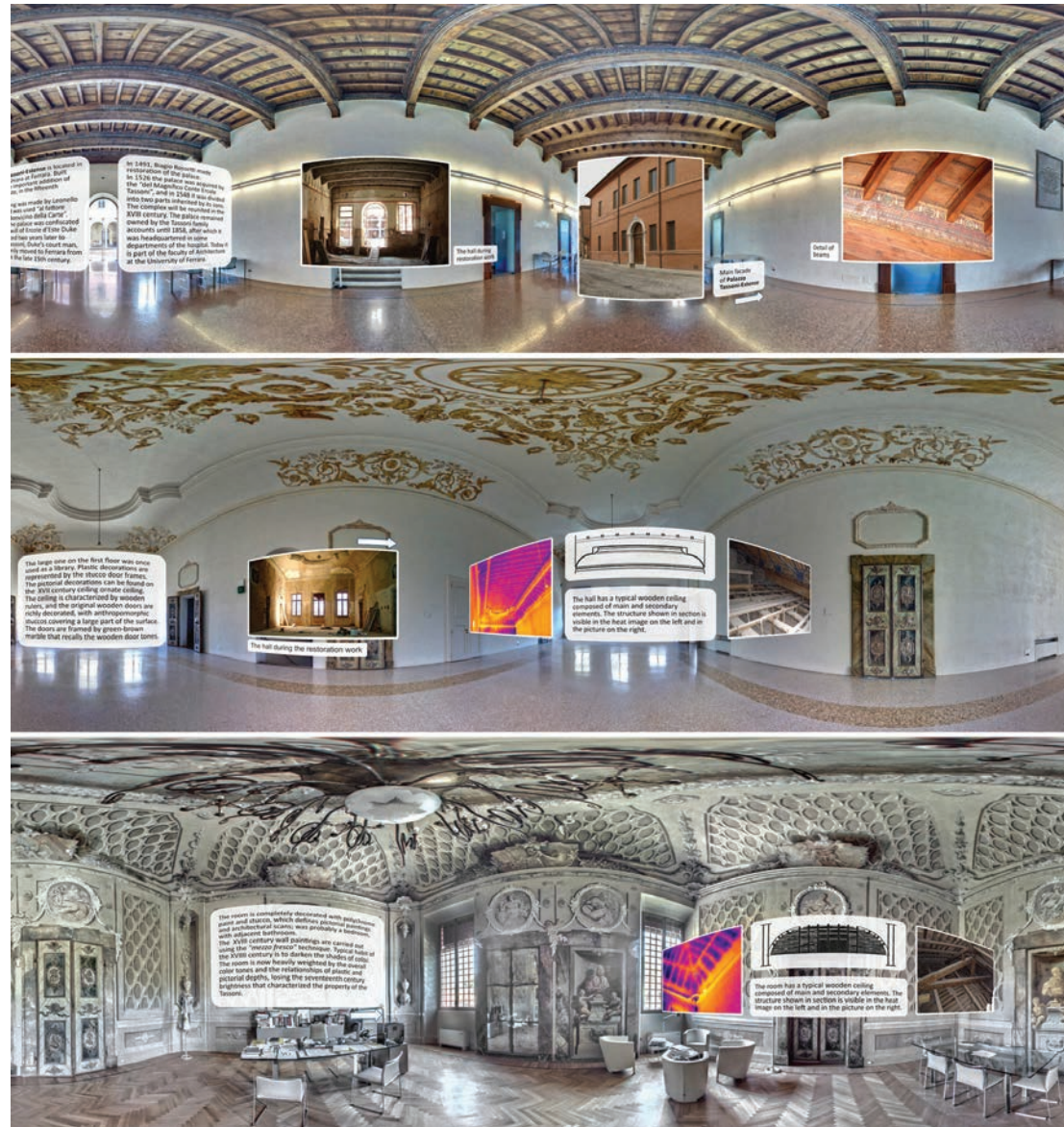
Fig. 3 - For the Tassoni-Estense Palace, an interactive tour has been realized, mainly using raster images in order to be easily used on-the-go (it doesn't require high CPU level or bandwidth) by web browsing and All-in-one HMD. The source data are 36 of the 123 spherical images captured during the survey campaign.
