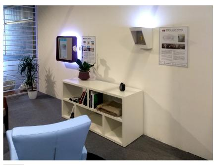
FIG. 5 The image shows the functioning prototypes of the HABITAT system: the digital 'frame' interface (top-left); smart chair; and indoor localization system inside the lamp (top-right). Source: M. Marchi, 2019
