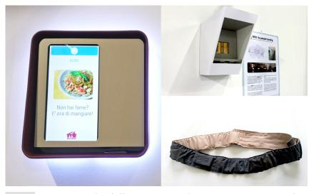
FIG. 3 The digital interface (left); the reader lamp of the indoor localization system (topright); the wearable inertial sensor for tracking elderly people's movements (bottom-right). Source: M. Marchi, 2018
