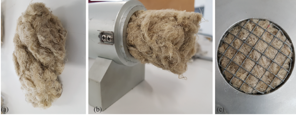
Figure 2: Investigated hemp fibres: a) loose hemp fibres; b) a fibrous material sample is created within the test rig; c) metallic mesh used to restrain the fibres in the sample holder.
