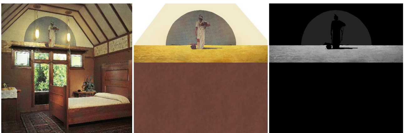
Fig. 4 - From left to right: reference photo (A. Abernathy, The Oak Park Home and Studio of Frank Lloyd Wright , 1988, p.21), example of mapping for the material's surface and example of mapping of the glossiness characteristic of the same surface
