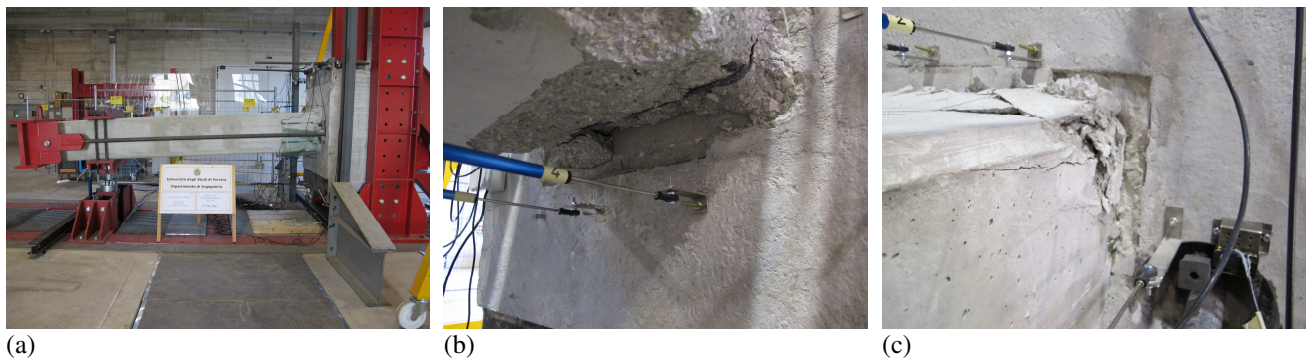
Fig. 9 (a) Column deflected configuration during the last half-cycle; and (b) bottom and (c) top sides of the column in proximity of the joint section at the end of test
