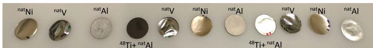
Fig. 2: Photograph of the stacked-foils target typically used in the PASTA project.
