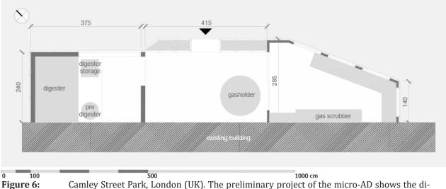
Camley Street Park, London (UK). The preliminary project of the micro-AD shows the dimenson of the technological components and the equipment designed. *Source: acknowledgment to Rokiah Yaman, Director of Community by Design, London, UK, for the material provided.*
