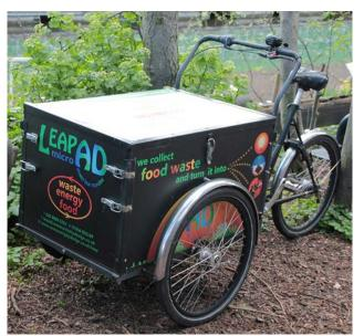
**Figure 7:** Camley Street Park, London (UK). Cargo bike is used for food waste collection direct to Camley Street Park anaerobic digester. The cargo collects 100 kg of food waste has a speed of 15/20 km/h and is used in an area of 3,2 km of radius. *Source: photo by Pracucci, 2017.*
