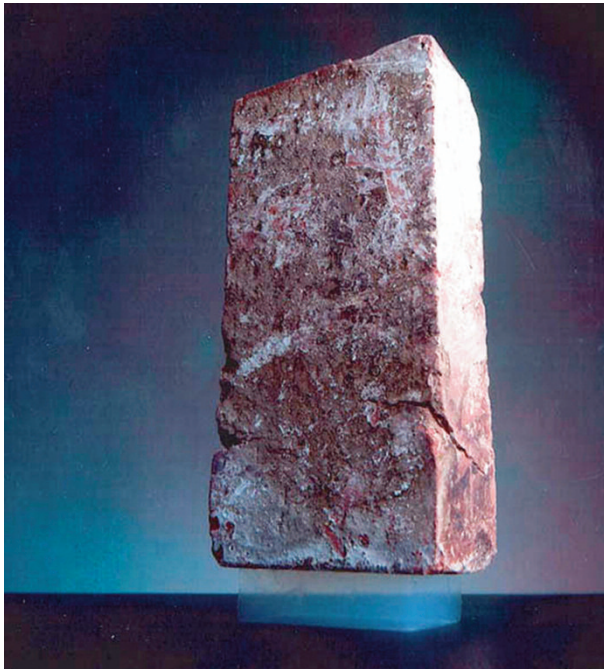
Fig. 6 - The Aerogel, discovered in 1931 but remained practically unknown until 1970s, has a density equal to three times that of air but it is able to support significant loads, being at the same time an excellent insulating material (credit: Addington and Schodek, 2005).
